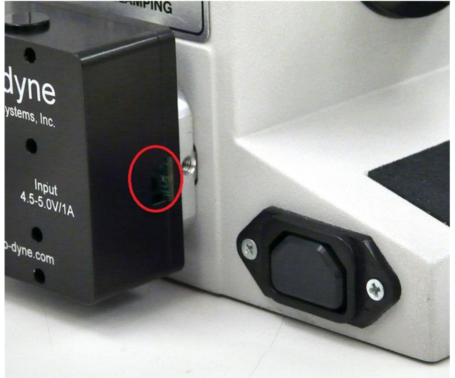
(2) Rubber AC blocking plug installed in obsolete AC receptacle.
