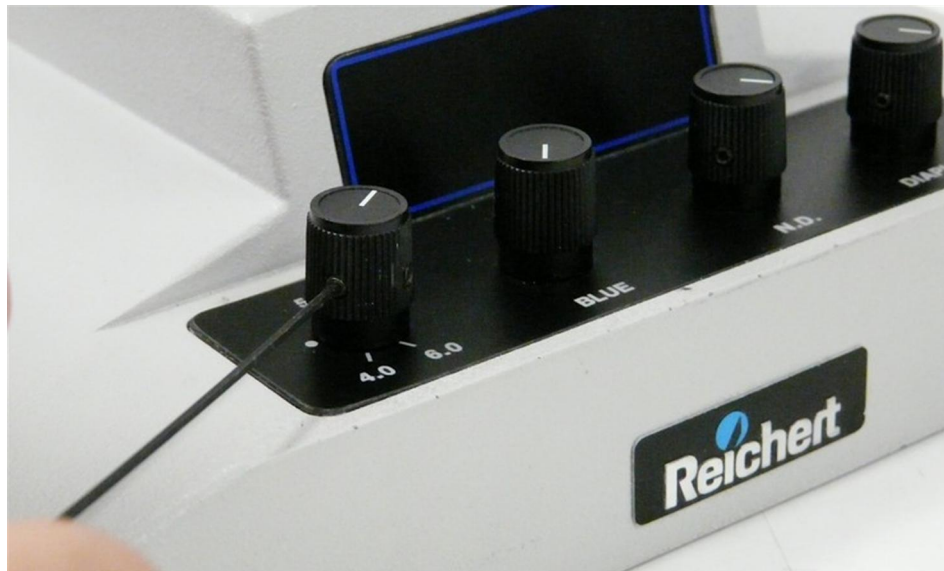
(4) Using the hex key provided, loosen the set screw holding the brightness knob on the old pot.
